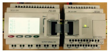
Repeat the expansion module steps to mount further expansion modules.
