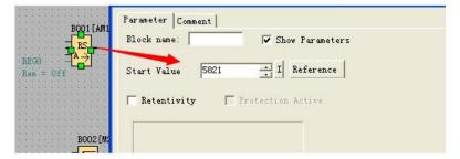
2. The HEG value of the data latch relay can be modified by press OK key for 3 seconds in text message block.
